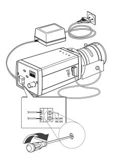
AC230V Power Input Camera Connect the power input cord to the AC 230V power source.
